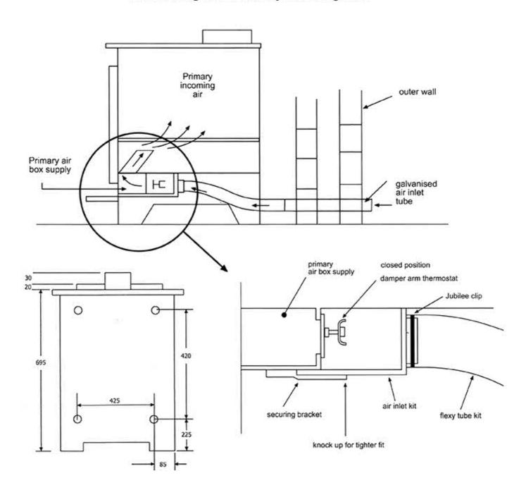
As building Regulations state at this moment, you must have permanent open air vent into the same room as your appliance. But with the addition of our Air Kit it helps to eliminate draughts because over 80% of the air required for the stove comes through the tube supplied with our kit. It will reduce the number of air changes in the room so significantly reduce the heat loss from the room & therefor wont pull air through the required air vents into the room.
