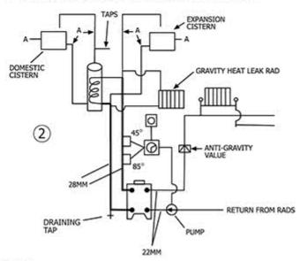
Remember that, although the built in thermostat can close the fire down, it cannot completely stop combustion - it is essential to supply some means of dissipating surplus heat, such as a permanently connected radiator or hot water system. The use of a leak stopper/corrosion inhibitor, such as Dunsley 'Oxypic' is highly recommended.
