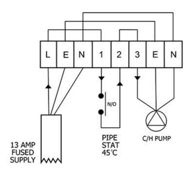
During summer months if heating is not required for radiators turn the pipe stat up to 80C to supply cylinder on gravity only.
